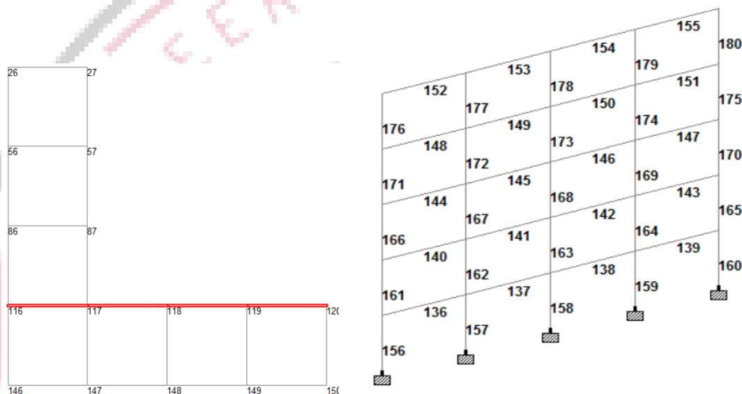
Figure 6 Beams and column numbering at section X-X
